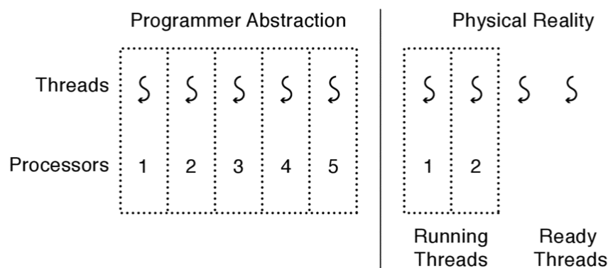
Figure 4.1: The operating system provides the illusion that programmers can create as many threads as they need, and each thread runs on its own dedicated virtual processor. In reality, of course, a machine only has a finite number of processors, and it is the operating system's job to transparently multiplex threads onto the actual processors.
