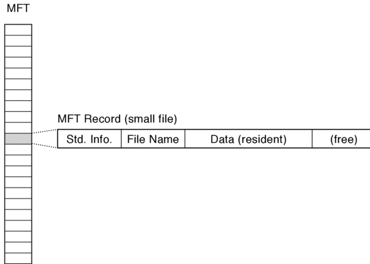
Figure 13.16: A small file's data can be resident , meaning that the file's data is stored in its MFT record.
