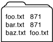
Figure 13.7: In this directory, the hard links foo.txt and bar.txt and the soft link baz.txt all refer to the same file.
